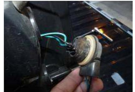
Step 5: Pull out the new Anzo tail light and locate the loose 1157 wedge connector. Plug this into the light bulb wire harness lining up the black wire to black and green to green.
