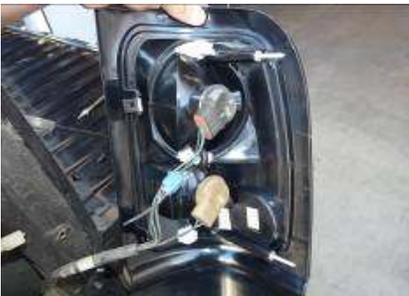
Step 6: Twist the light bulb wire harness into the new Anzo light.
